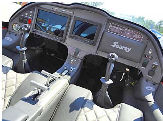
Searey Elite features a modern glass instrument panel. The SLSA model might one day offer an adjustable pitch prop; experimental models could offer it even sooner, if builder/customers wish.
