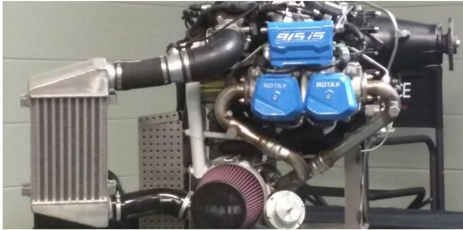
***A mockup of the Rotax 915iS with a turbocharger and intercooler, as well as a larger gearbox
